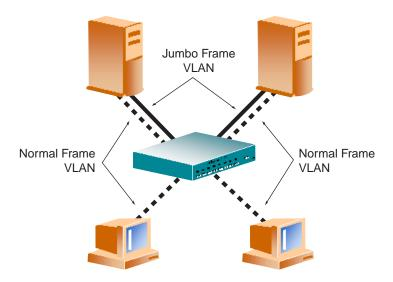
Figure 2-7 Jumbo Frame VLANs
